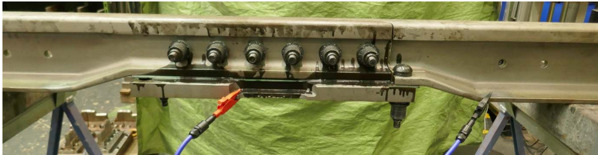
Figure 5: Measurement of insulation resistance between footplate and one rail profile
