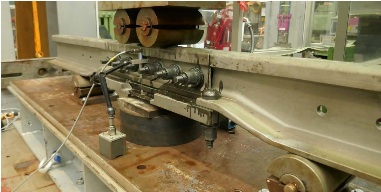
Figure 4: Sample ABJ-009 in the test set-up of the bending fatigue test
